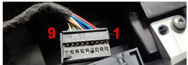
c) Loosen the plug of the instrument cluster and remove the outer housing of the connector. Now carefully remove approx. 10cm of the cable sheath.
