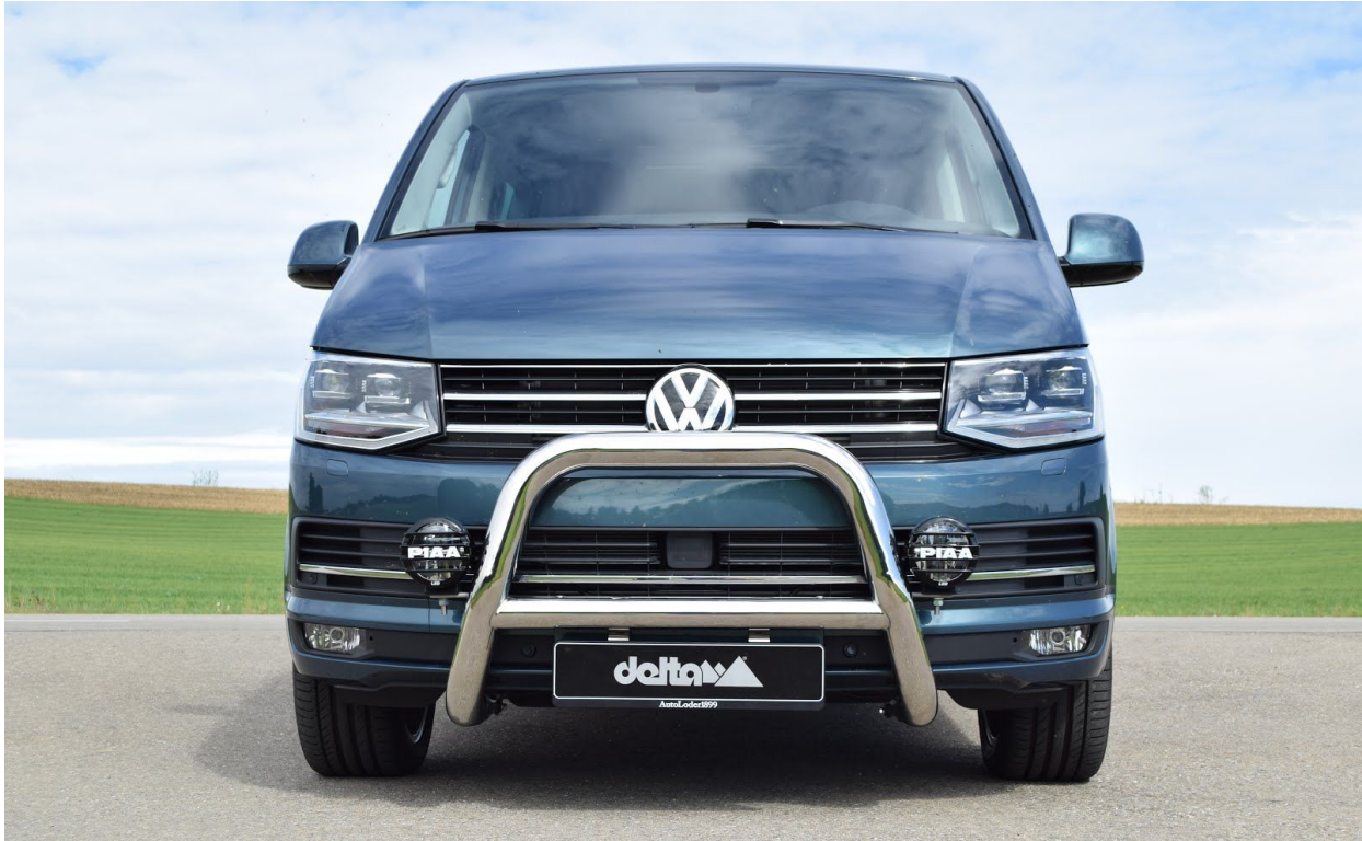
Picture shows frontbar without underride protection and with extra lights
